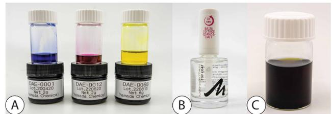
Figure 4: The Photochromic Mixture. (A) cyan, magenta and yellow photochromic dyes, individually mixed with transparent nail polish. (B) Transparent nail polish. (C) Fully saturated mixture of transparent nail polish and CMY dyes.
